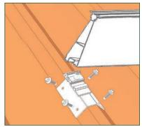
• Mount the Fix2000 with KlickTop connector with consideration to the shade distance to modules rows.
